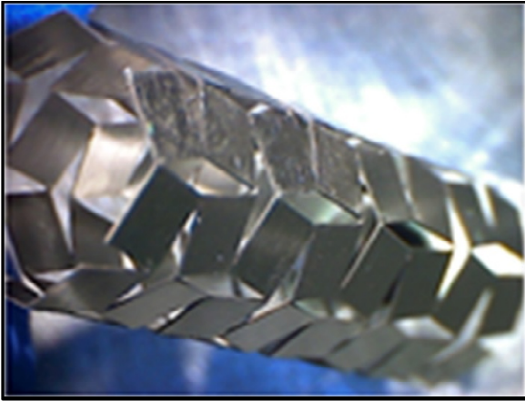
Fig. 5. Auxetic stent with drug delivery system, [90].
