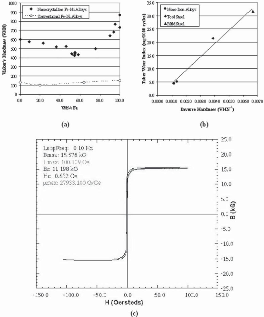
**Fig. 2.** (a) Vickers hardness as a function of iron content for various conventional and nanocrystalline Fe-Ni alloys, (b) Taber Wear Index as a function of inverse Vickers hardness for nanocrystalline Fe and conventional iron alloys, and (c) A B-H Loop measured at 0.1 Hz for nanocrystalline Fe-42wt%Ni in the as-deposited condition.
