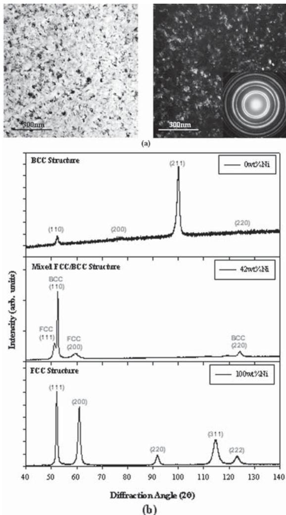
**Fig. 1.** (a) Bright and dark field TEM micrographs and the corresponding selected area diffraction pattern (inset) of electrodeposited nanocrystalline Fe-42wt%Ni, and (b) X-Ray diffraction patterns of electrodeposited Fe-Ni alloys with various Fe concentrations.
