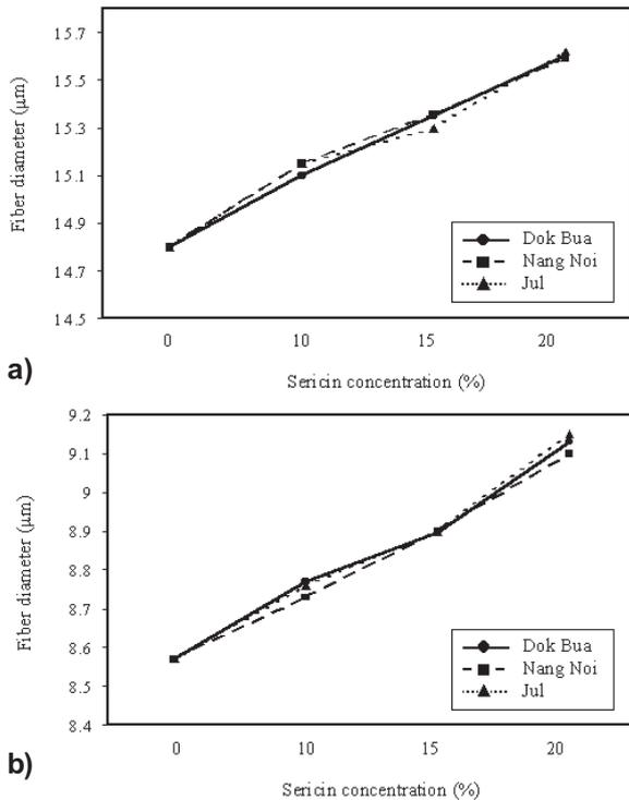
Fig. 3. The fiber diameter of: (a) nylon fiber and (b) polyester fiber coated with sericin.
