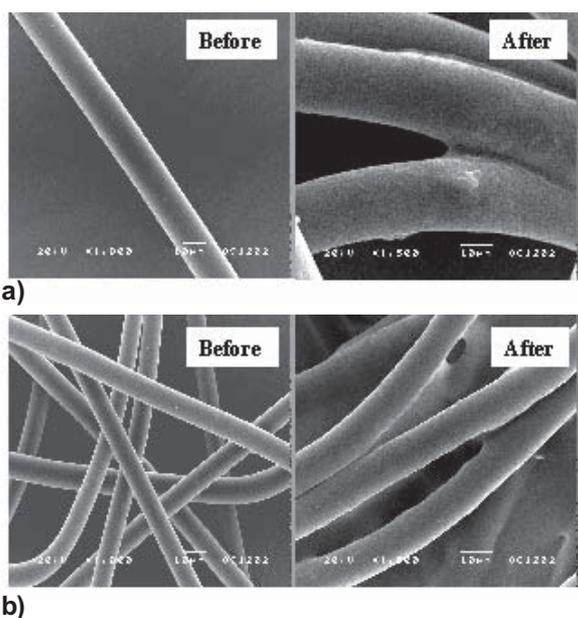
**Fig. 2.** The morphology of: (a) nylon fiber and (b) polyester fiber coated with sericin.
