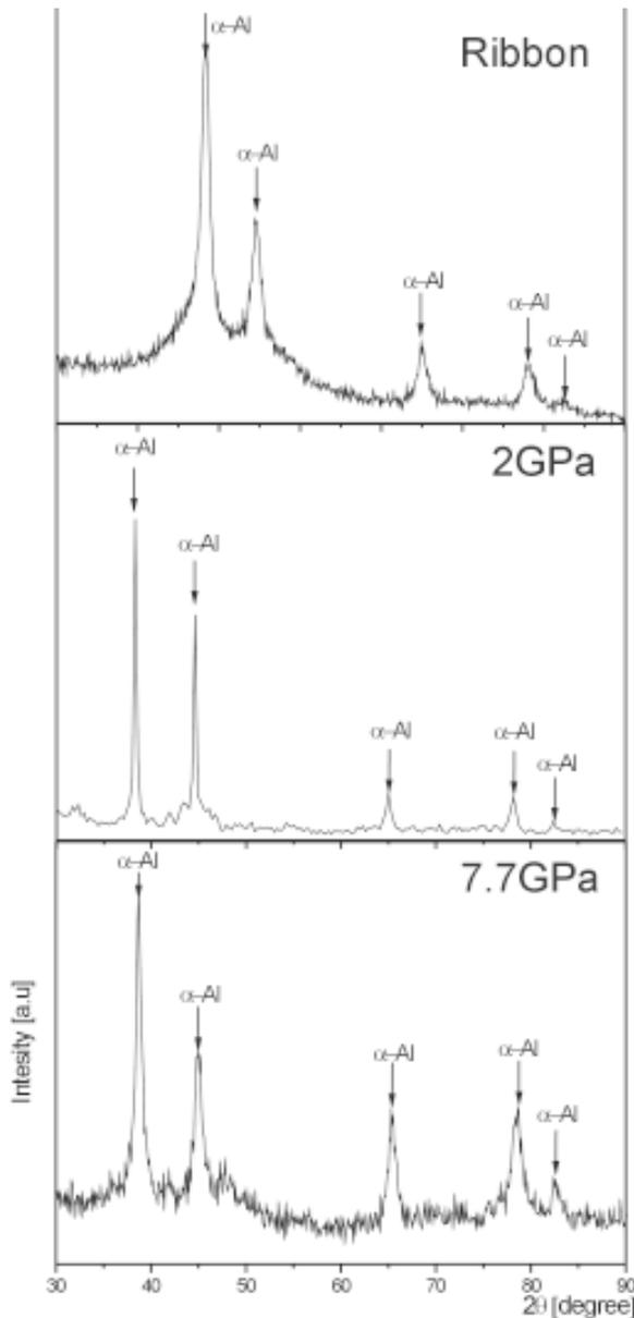
**Fig. 1.** XRD patterns of melt spun ribbon (a), bulk sample compacted at 2 GPa (b) and at 7.7 GPa (c).
