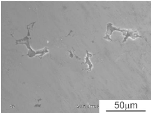
**Fig. 4.** SEM micrograph of the surface of the bulk sample compacted at 4 GPa and 200 °C.
