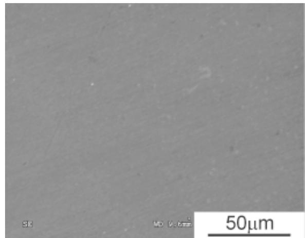
**Fig. 6.** SEM micrograph of the surface of the bulk sample compacted at 7.7 GPa and 200 °C.
