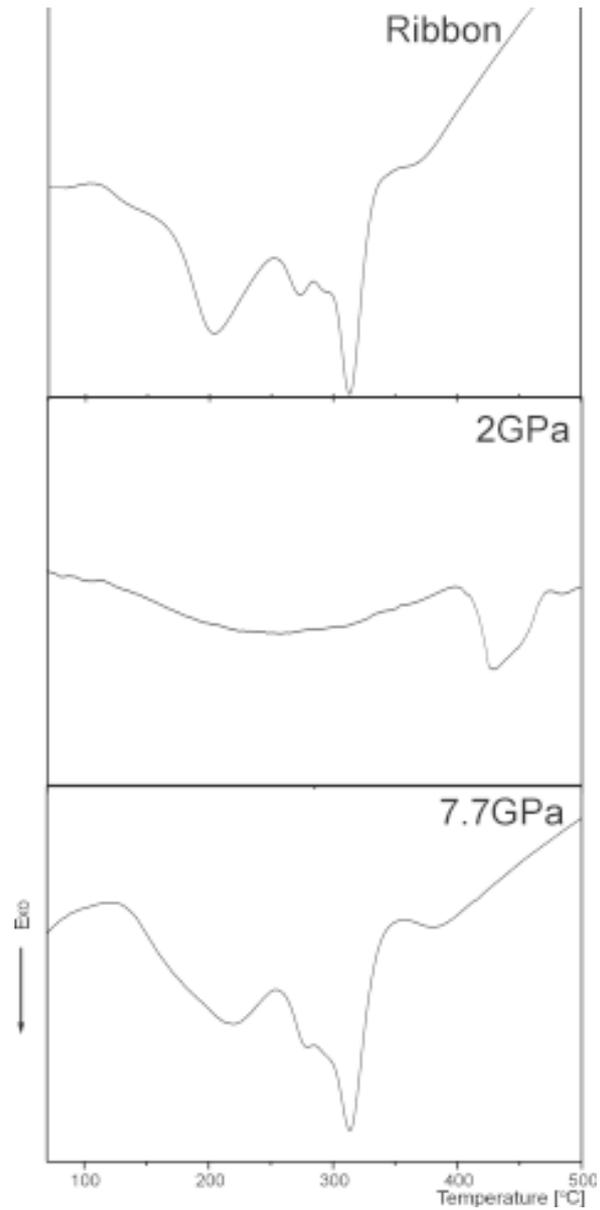
**Fig. 2.** DSC traces of the melt spun ribbon (a), bulk sample compacted at 2 GPa (b) and at 7.7 GPa (c).
