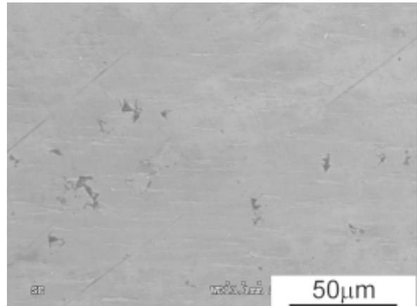
**Fig. 5.** SEM micrograph of the surface of the bulk sample compacted at 6 GPa and 200 °C.
