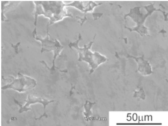
**Fig. 3.** SEM micrograph of the surface of the bulk sample compacted at 2 GPa and 200 °C.
