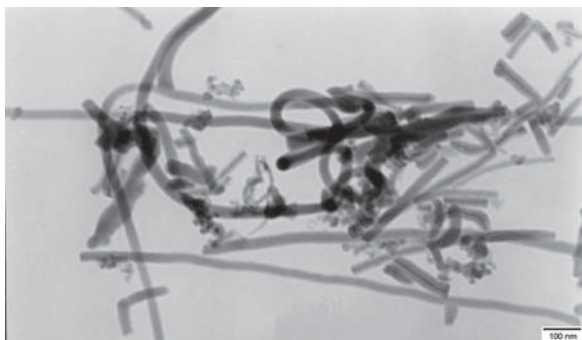
Fig. 8. TEM image of filled CNT and nanofibers from calcined sucrose and graphite sample heated 60 min without catalyst.
