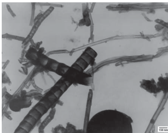
Fig. 10. TEM image of a CNT and a multi-walled bamboo-like structure in Boric Acid graphite heated 180 min without catalyst.
