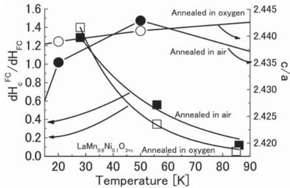
**Fig.3.** The temperature dependence of  $dH_c^{FC}/dH_{FC}$  and  $c/a$ .
