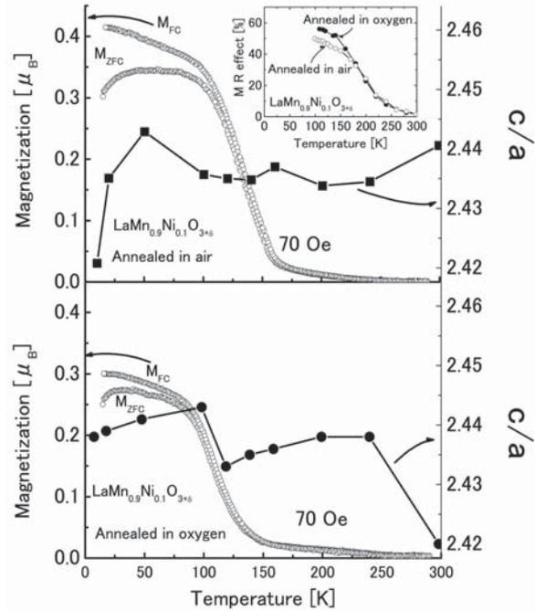
**Fig.1.** The temperature dependence of  $M_{ZFC}$ ,  $M_{FC}$  and  $c/a$  in  $\text{LaMn}_{1-x}\text{Ni}_x\text{O}_{3+\delta}$  annealed in air (upper graph) or oxygen atmosphere (lower graph). The inset (upper graph) is the temperature dependence of MR effect.
