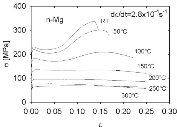
Fig. 1. Stress strain curves obtain for various temperatures.
