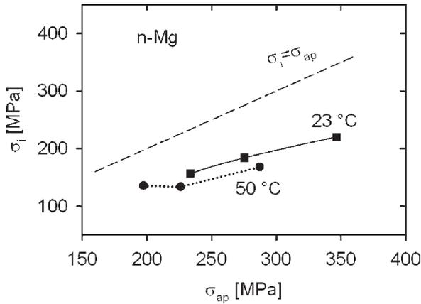
**Fig. 3.** Internal stress obtained at two temperatures.
