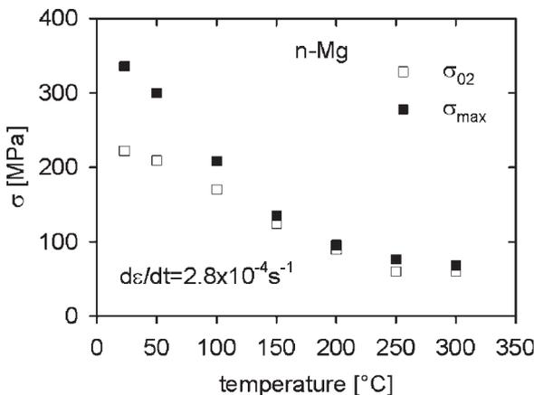
**Fig. 2.** Temperature dependence of the yield stress as well as the maximum stress.
