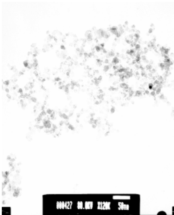
Fig. 1. TEM photograph of \text{Al}_2\text{O}_3 nanoparticle.
