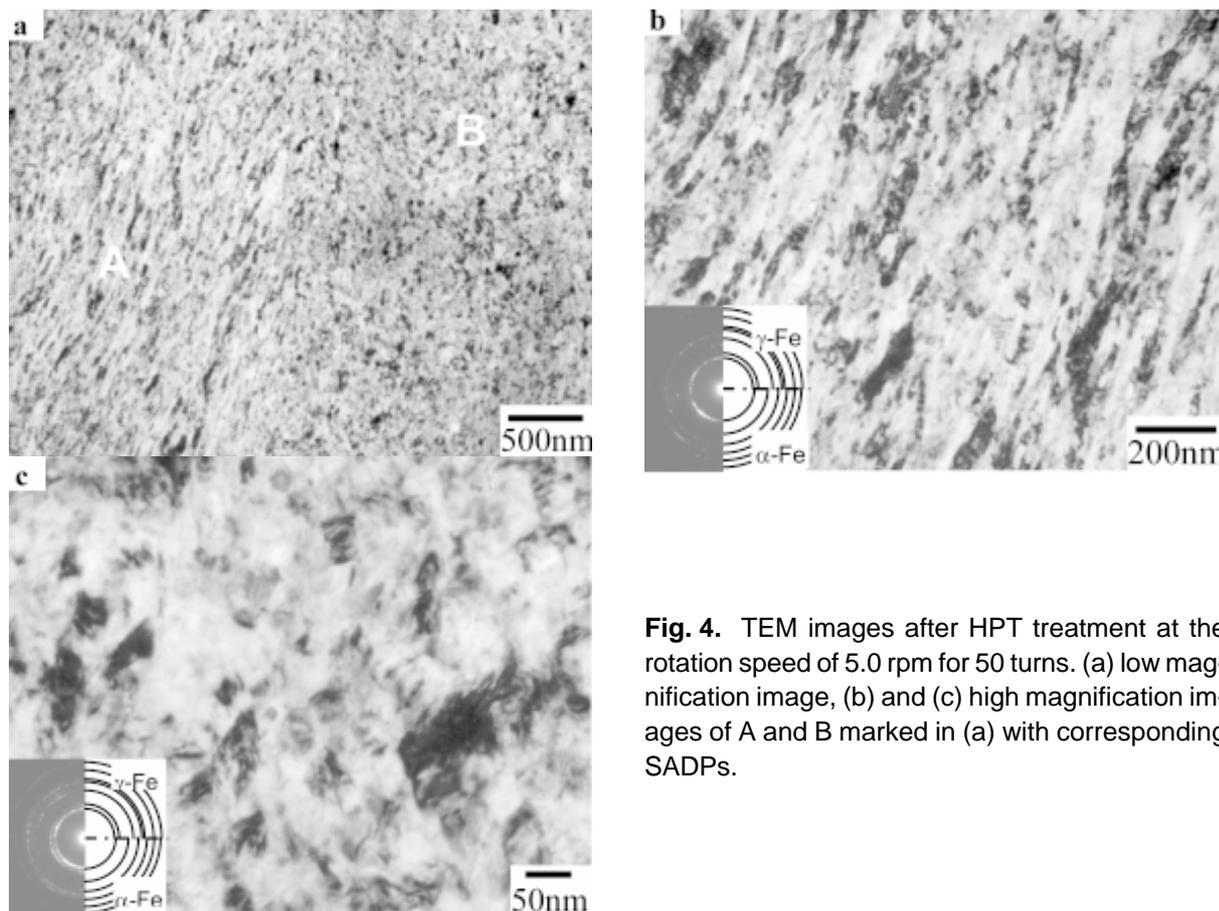
**Fig. 4.** TEM images after HPT treatment at the rotation speed of 5.0 rpm for 50 turns. (a) low magnification image, (b) and (c) high magnification images of A and B marked in (a) with corresponding SADPs.
