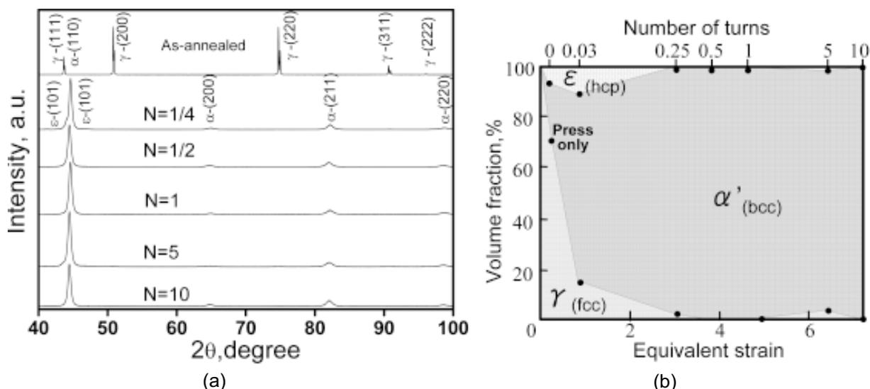
**Fig. 1.** X-ray spectra and volume fractions of composed phases in the specimens before and after HPT at rotation speed of 0.2 rpm. (a) X-ray spectra, (b) volume fractions of composed phases.
