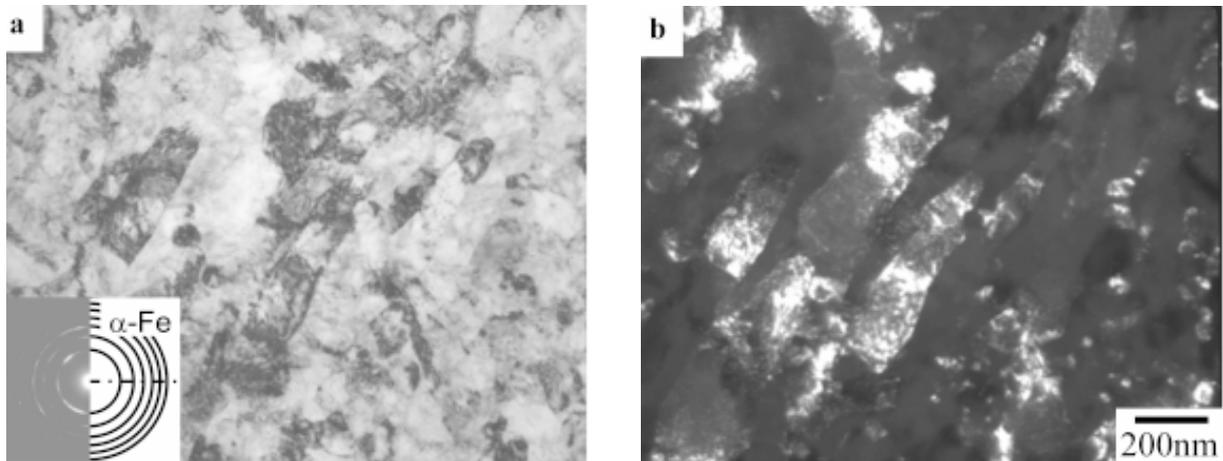
**Fig. 3.** TEM images after HPT treatment at the rotation speed of 0.2 rpm for 10 turns. (a) bright field image and corresponding SADP, (b) corresponding dark field image.
