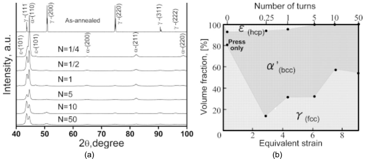
**Fig. 2.** X-ray spectra and volume fractions of composed phases in the specimens before and after HPT at rotation speed of 5.0 rpm. (a) X-ray spectra, (b) volume fractions of composed phases.
