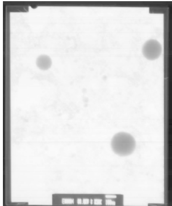
Fig. 3. TEM picture of uniformly dispersed TiO 2 particles after the particle dispersion treatment.
