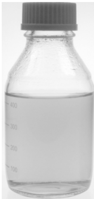
Fig. 3. The sample of Ag nanoparticles suspended in pure water (pale yellow color).
