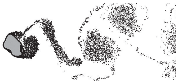
Figure 1: Vortex wake around the iced conductor cross-section
