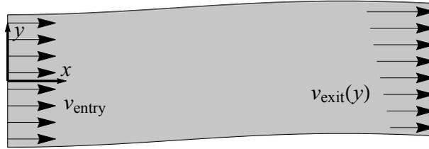
Figure 1: Deformation of a plate with prescribed velocities at the boundaries
