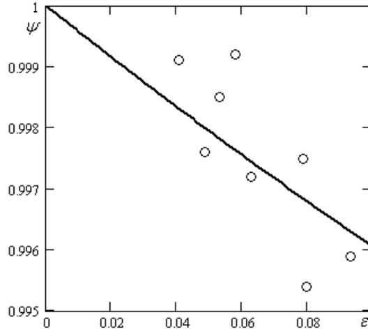
Figure 3: Theoretical curves of density changes (solid line) for  $\alpha = 6$  and experimental points of density changes of pure copper during creep under  $500^\circ C$  [8] (circle points).
