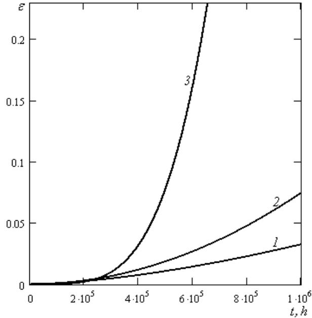
Figure 5: The theoretical creep deformation curves according to the relation (9) for different values of the coefficient  $\alpha$ :  $\alpha = 6$  - curve 1,  $\alpha = 4$  - curve 2 and  $\alpha = 2$  - curve 3.
