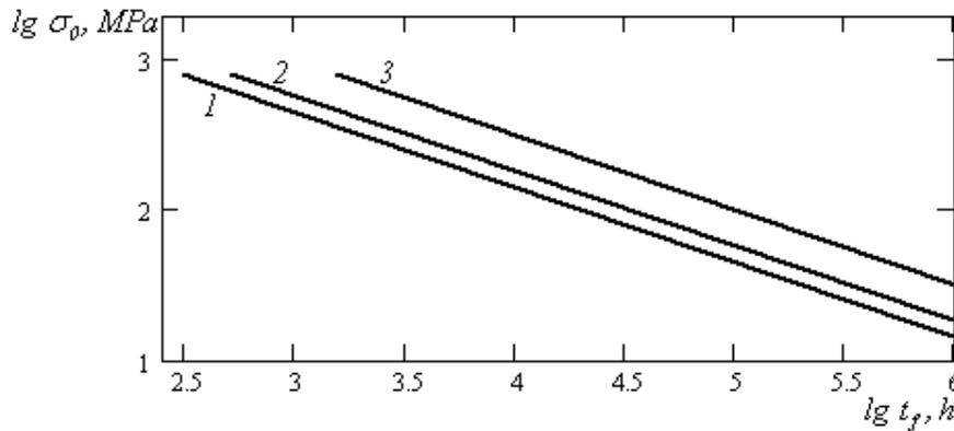
Figure 4: Curves of long-term strength under criterion (12):  $\alpha = 6$  - curve 1,  $\alpha = 4$  - curve 2 and  $\alpha = 2$  - curve 3.
