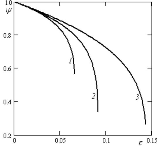
Figure 2: The curves  $\psi(\varepsilon)$  according (11) for different values of parameter  $\alpha$ :  $\alpha = 6$  - curve 1,  $\alpha = 4$  - curve 2 and  $\alpha = 2$  - curve 3.
