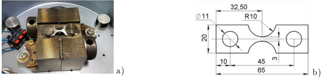
Figure 1: a) Installation for carrying out experiments on thermal fatigue, b) Geometry corset sample for thermal fatigue experiment.
