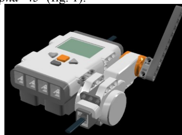
Fig. 1. Motor stabilizing in position 45^\circ .
