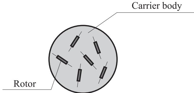
Figure 2: Multi-rotor gyrostat
