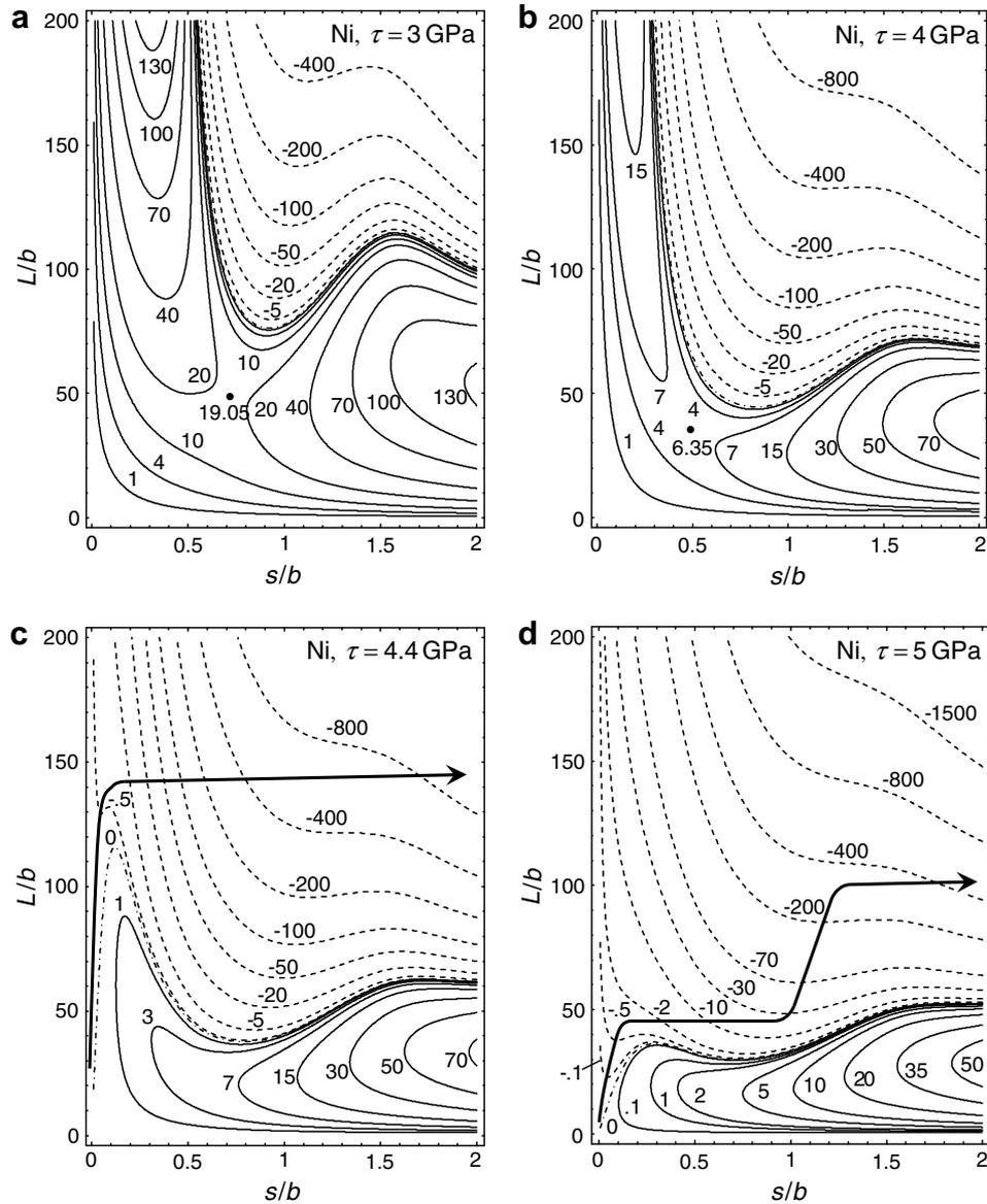
Fig. 4. Maps of the energy change  $\Delta W(x, y)$ , where  $x = s/b$  and  $y = L/b$ , for pure Ni under the external shear stress (a)  $\tau = 3$  GPa, (b) 4 GPa, (c) 4.4 GPa and (d) 5 GPa. The values of  $\Delta W$  are given in electron-volts. The bold dots in maps (a, b) show the saddle points. The thick arrowed curves in maps (c, d) approximately image the barrier-less evolution of a dislocation loop in strength and size.
