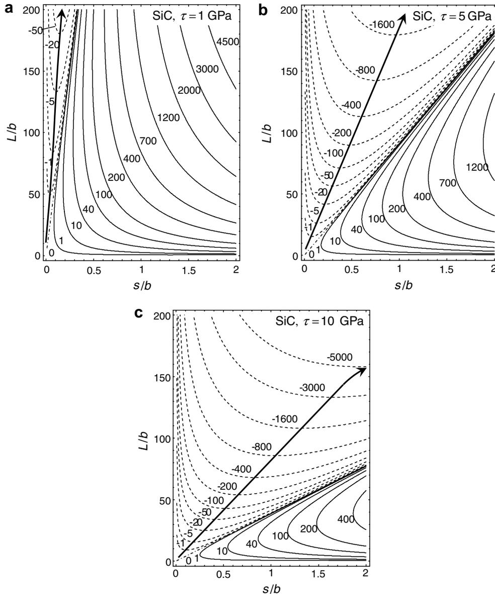
Fig. 5. Maps of the energy change  $\Delta W(x, y)$ , where  $x = s/b$  and  $y = L/b$ , for 3C-SiC under the external shear stress (a)  $\tau = 1$  GPa, (b) 5 GPa and (c) 10 GPa. The values of  $\Delta W$  are given in electron-volts. The thick arrowed curves approximately image the barrier-less evolution of a dislocation loop in strength and size.
