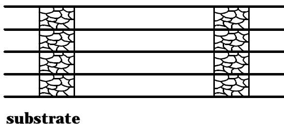
Fig. 22. Coatings with spatially variable structures containing single crystalline and nanocrystalline regions.
