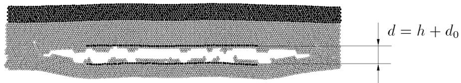
Figure 2: Measuring of the width of the spall crack.
