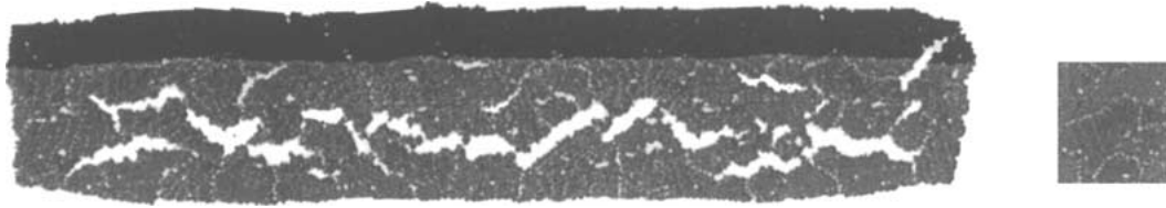
Figure 10. Spallation in polycrystal target. The rectangle shows an element of the original target material (1% porosity).
